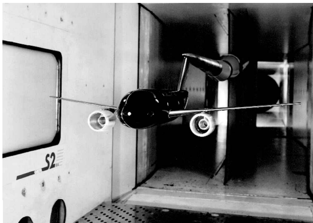
Fig. 1 DLR-F6 model with VHBR nacelles in the ONERA S2MA wind tunnel.
